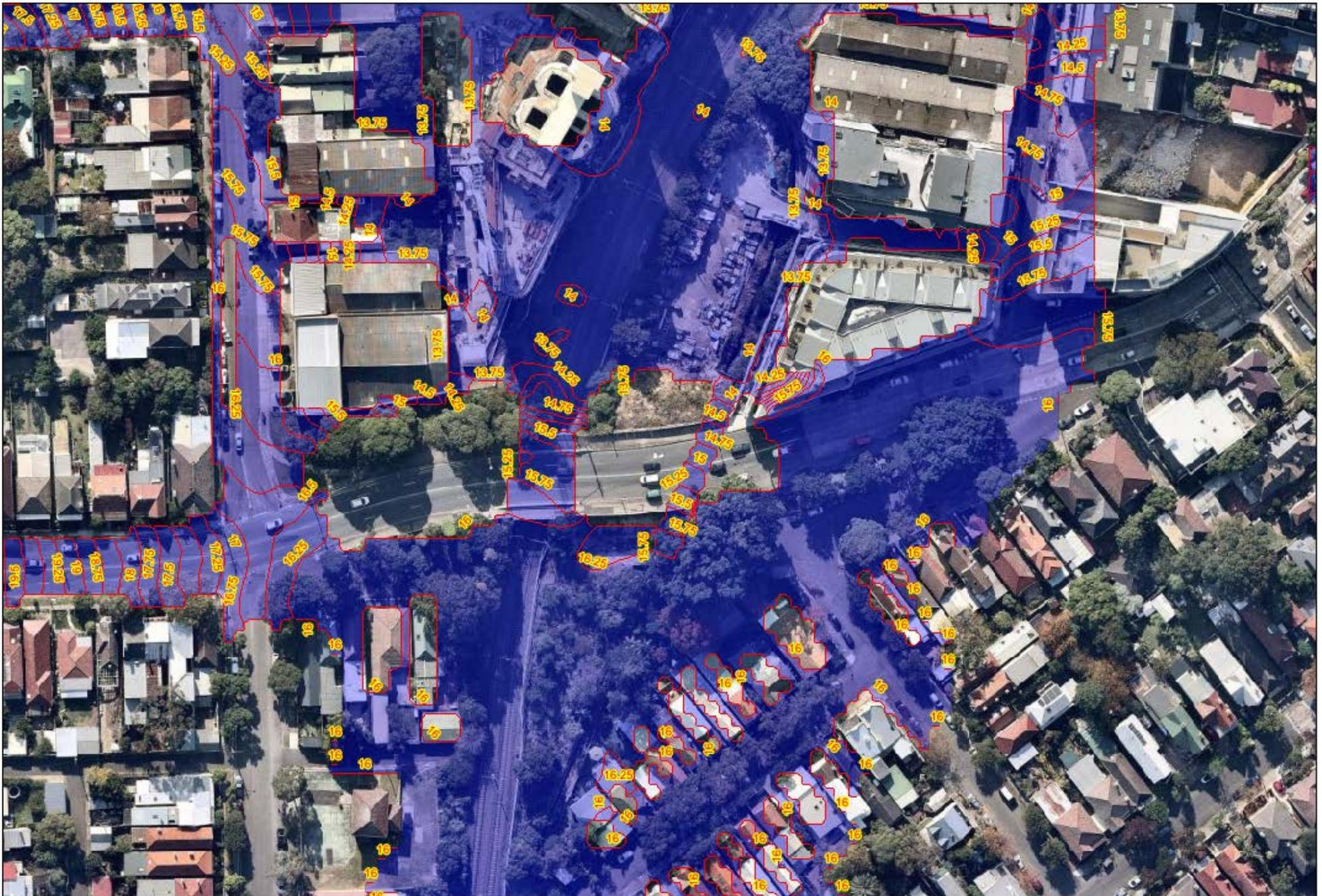
Figure 12 PMF Extents and Flood Levels (m AHD) – Benchmark Conditions
