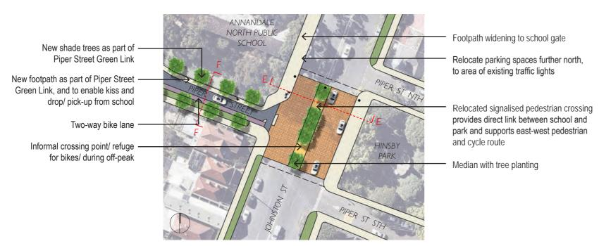
FIGURE 21: JOHNSTON STREET AND PIPER STREET INTERSECTION (not to scale)
