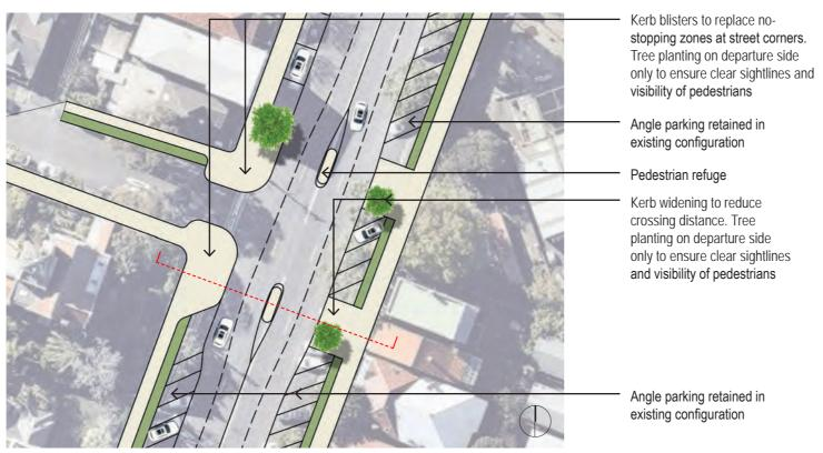
FIGURE 20: TYPICAL PLAN STREETSCAPE TYPE 3 - KERB WIDENING AT INTERSECTIONS (not to scale)
