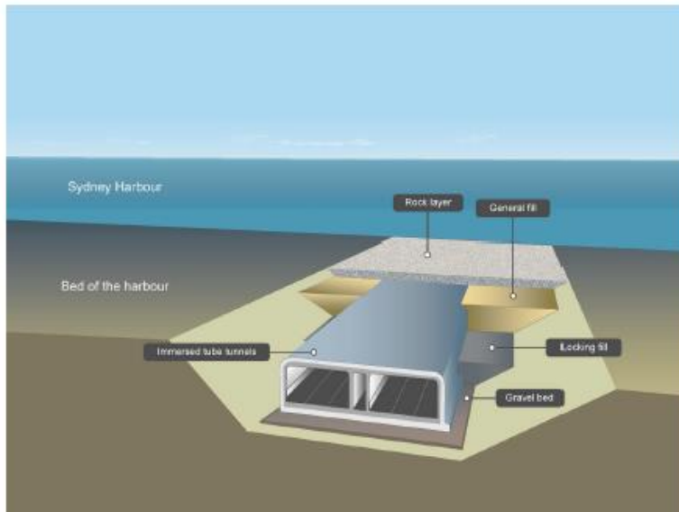
Figure 6-18 Example of an immersed tube tunnel
