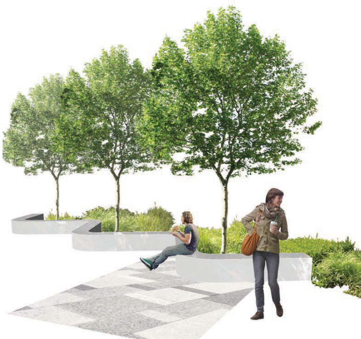
Custom concrete seating wall- accommodates individuals and groups. The articulated form also allows for protected spaces for planting and street trees- see below for plan and see pages 61- 62 for potential feature tile treatments to selected seating elements
