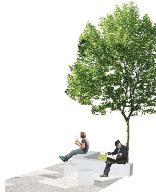
Custom concrete seating wall- 'outward corner'. The articulated form also allows for 'inward' or 'outward' seating arrangements- see below for plan and see pages 61- 62 for potential feature tile treatments to selected seating elements
