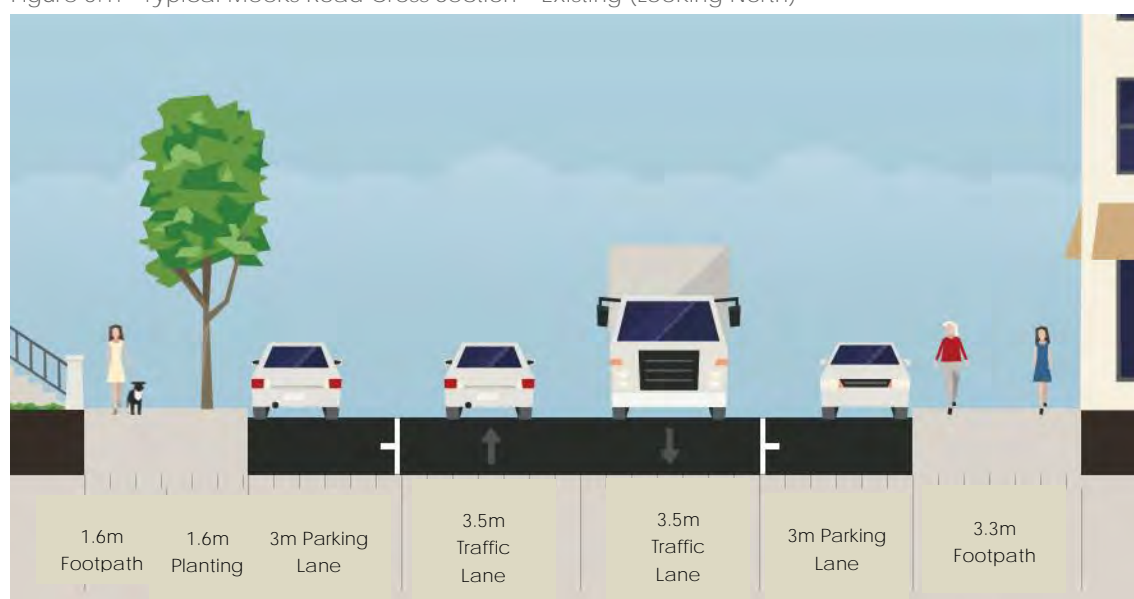
Figure 5.2: Typical Lord Street Cross Section – Existing (Looking West)
