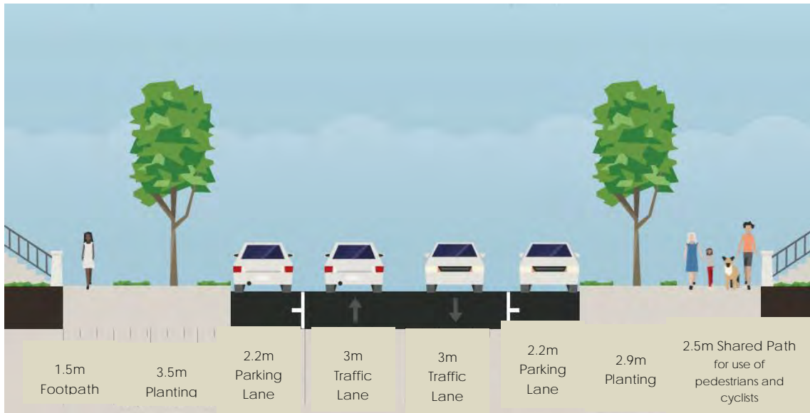
Figure 5.3: Typical Edwin Street Cross Section – Proposed (Looking North)
